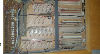
within our organ are wrapped in cotton, not coated with plastic or printed on a circuit board. As electricity flows through these wires, there's a risk of fire or short circuit.
